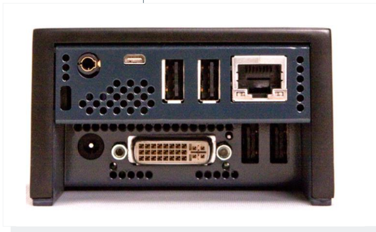
Figure 8: Ports and connectors on the rear of the Pano Zero Client.
